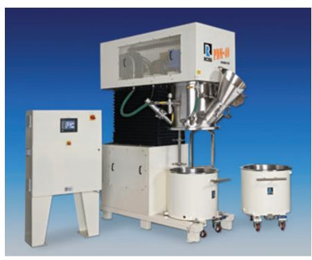
Planetary disperser with a 40-gal capacity, designed for viscosities up to around 2 million cP.
