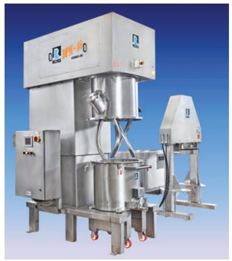
Double-planetary mixer with discharge system, in all-stainless steel construction, designed for production of hydrogel adhesives used in sterile wound dressings. The helical blades handle ultra-high viscosities up to around 6 million cP.
